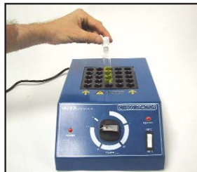
2: Place the vial in the reactor and set the timer.
