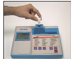
3: Place the vial in the Hanna C 99 and read the results.
